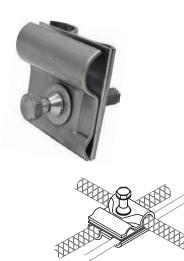
The universal clamp connector for connection type T-joint, cross joint and parallel join between rebar to rebar, rebar to round conductor, round conductor to round conductor. The shear bolt provide quick installation and the superior of connection.
