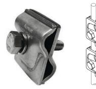
Universal Connector is made of Stainless Steel. There are two types of connecting process cross joint and parallel joint. The contact resistance shall be less than 1 m $\Omega$ , as well as the connected conductors tensile force s hall be more than 900 N
