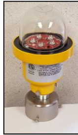
POL-21005-1B-R-SF-S SINGLE OBSTRUCTION LIGHT WITH 60MM SLIPFITTER FITS 2-3/8-INCH TENON
