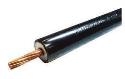
KHV Cable with a voltage-controlled sheath is typically used as an isolated down conductor in the field of lightning protection for control the separation distance according to IEC 62305-3
