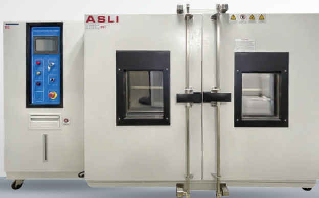
TEMPERATURE (HUMIDITY) Test Chamber
