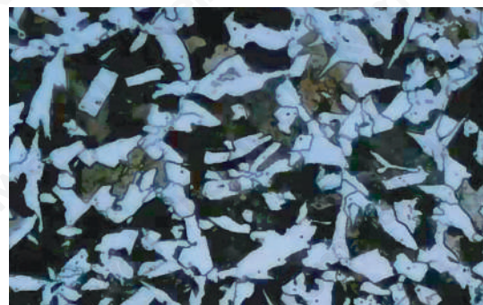
Macrostructure of a cross-section of exothermic welding for railway signaling bond
