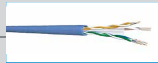
60088 UC 400 Cat 6 UTP 23 AWG PVC, IEC 60332-1 60075 UC 400 Cat 6 UTP 23 AWG LSZH, IEC 60332-1 62488 UC 400 Cat 6 UTP Bronze 24 AWG PVC, IEC 60332-1 62475 UC 400 Cat 6 UTP Bronze 24 AWG LSZH, IEC 60332-1 60048 UC 400 Cat 6 UTP 23 AWG LSFRZH, IEC 60332-3-24 60034 UC 400 Cat 6 UTP 23 AWG PE, Outdoor
