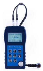
The ultrasonic thickness gauge Model **SW6** is featured as cost-efficiency and designed to make accurate measurements on steel, cast iron, aluminum, red copper, zinc, quartz glass, polyethylene, PVC, gray cast iron and nodular cast iron. Thickness measurements are made from one side of the material with no need to cut the part.
