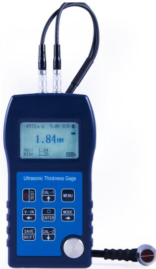
The ultrasonic thickness gauge Model **SW6** is featured as cost-efficiency and designed to make accurate measurements on steel, cast iron, aluminum, red copper, zinc, quartz glass, polyethylene, PVC, gray cast iron and nodular cast iron. Thickness measurements are made from one side of the material with no need to cut the part.
