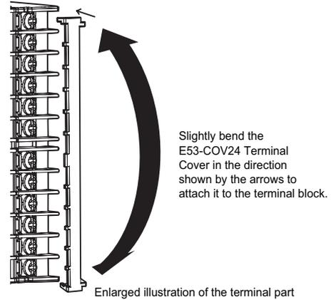
Slightly bend the E53-COV24 Terminal Cover in the direction shown by the arrows to attach it to the terminal block.
