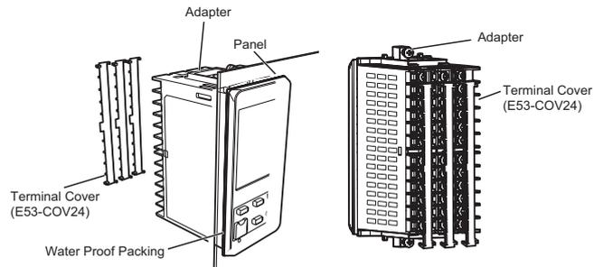
1. For waterproof mounting, waterproof packing must be installed on the Digital Temperature Controller. Waterproofing is not possible when group mounting several Digital Temperature Controllers. Waterproof packing is not necessary when there is no need for the waterproofing function.
