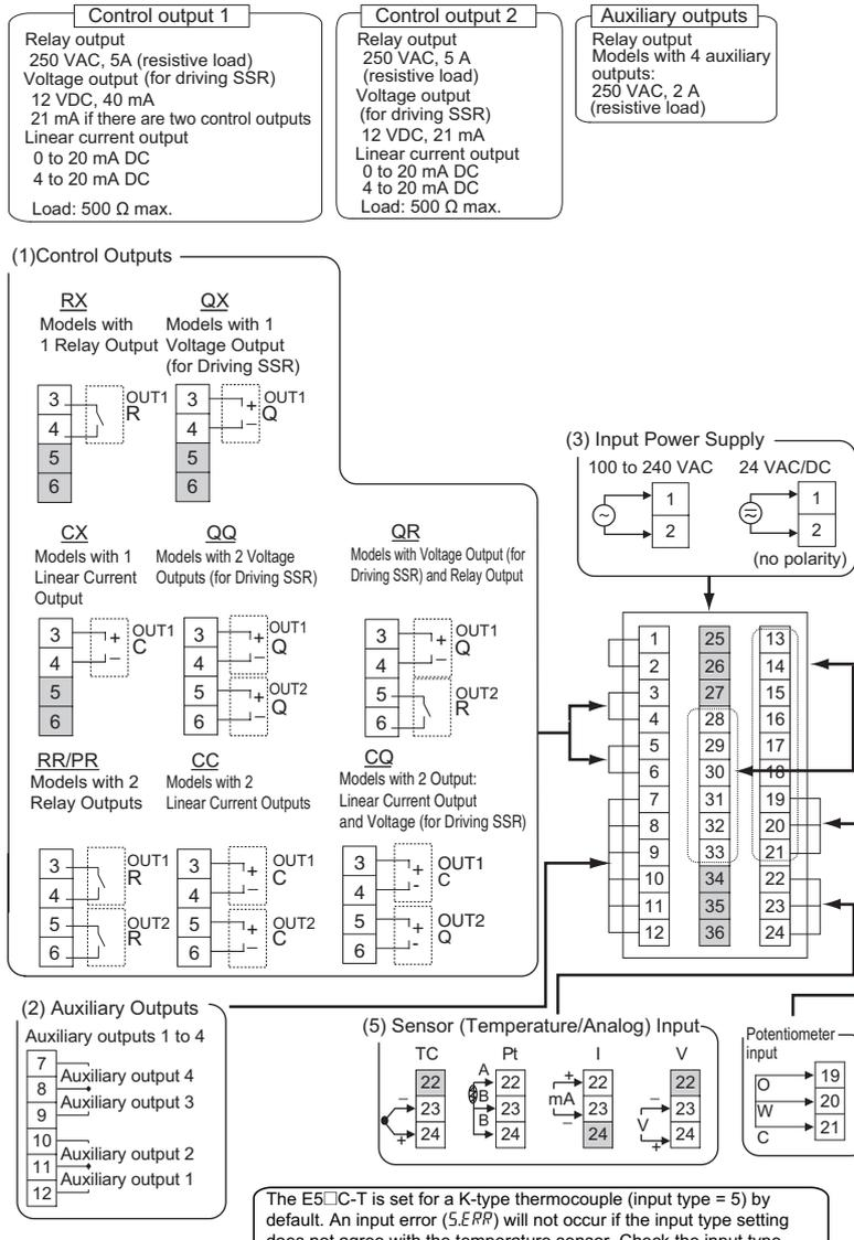
The E5□C-T is set for a K-type thermocouple (input type = 5) by default. An input error (5.ERR) will not occur if the input type setting does not agree with the temperature sensor. Check the input type.
