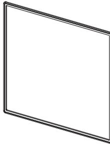
The Waterproof Packing is provided with the Temperature Controller.
