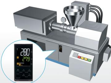
Heating/cooling control: Independent PID control
