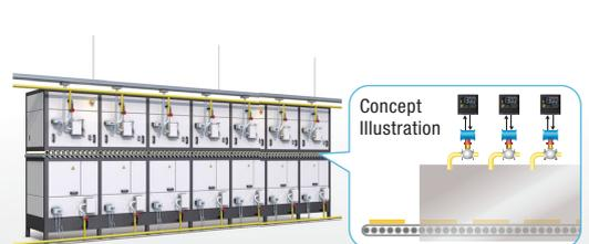
Motor-operated valve control: Position-proportional control
