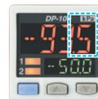
Displays measurements in 0.1 kPa
