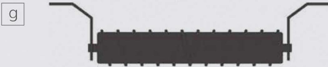
Spiral Return roller used to clean from materials that adhere to the belt. It's produced in spiral rubber.
