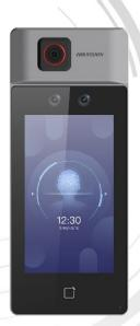
DS-K1T671TM-3XF face recognition terminal is a kind of access control device integrated with temperature screening function. It can fast take temperature and upload abnormal temperature event to the center, which can be widely applied in multiple scenarios, such as enterprises, stations, dwellings, factories, schools, campus and so on. Note that the device is not for medical use.
