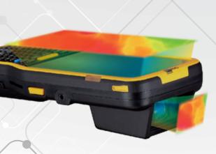
Comes with temperature sensor and heater control software allows user to automatically turn on/off heater based on surrounding environment. For example, set to turn on heater under -10°C and turn off above 20°C.
