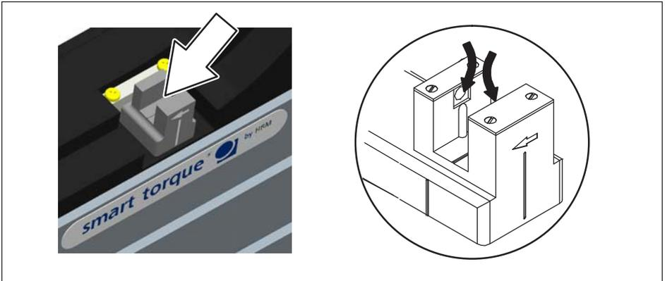
Fig. 15.1 *Cleaning points on the rotational speed sensor*
