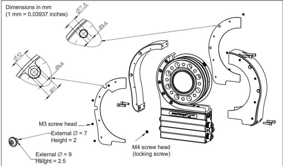
**Protection against contact plates 5 kN-m ... 10 kN-m**
