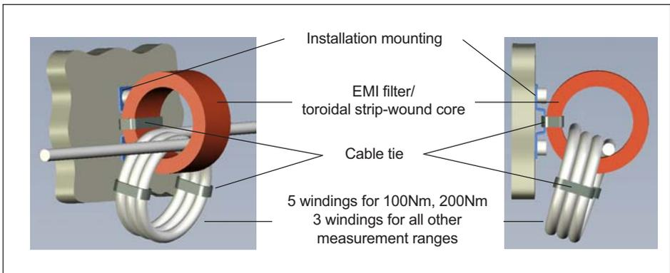
Fig. 10.1 EMI filter/toroidal strip-wound core installation example
