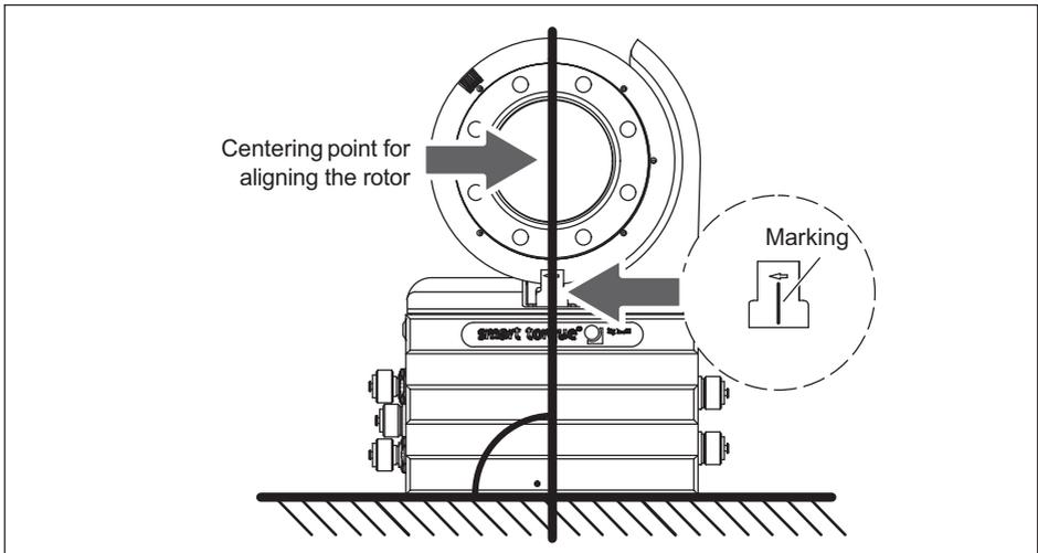
Fig. 8.22 Alignment markings on rotor and stator
