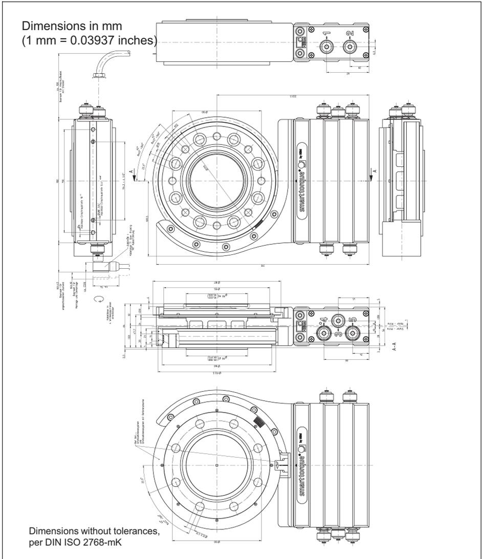
**Complete measurement flange, T12HP/10 kNm, with rotational speed measuring system**
