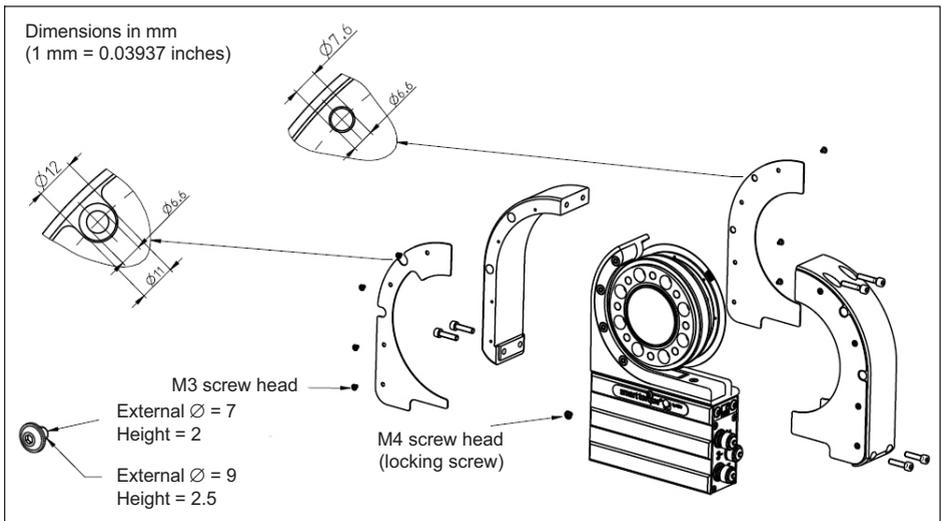
**Protection against contact plates 2 kN-m ... 3 kN-m**
