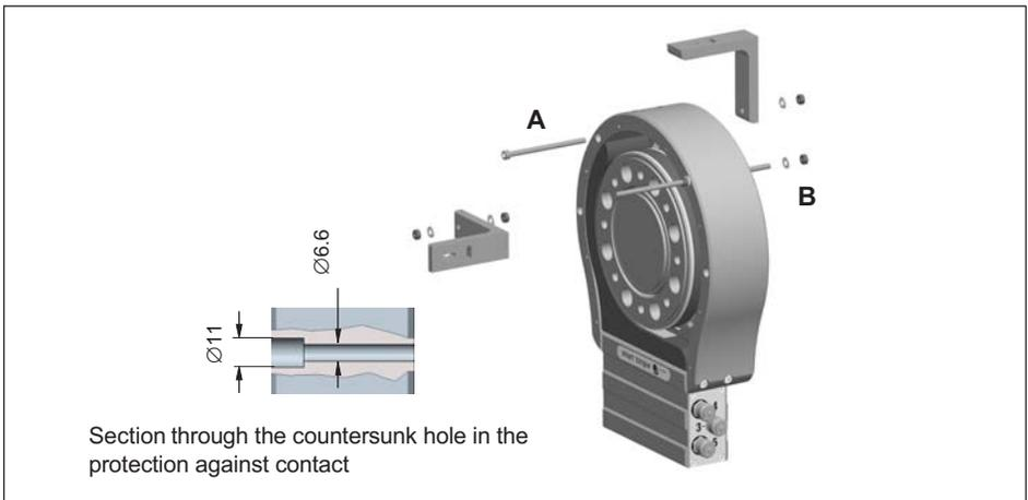
Fig. 8.14 Supporting the stator with protection against contact
