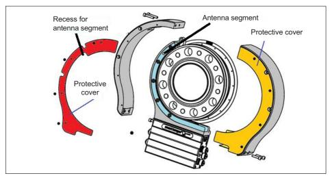
Fig. 8.8 Protective cover T12HP
