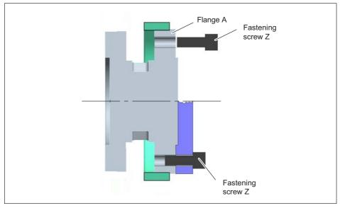
Fig. 8.3 Screw connections, flange A
