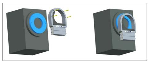
Fig. 8.20 Face-mounting on the customer side engine shielding
