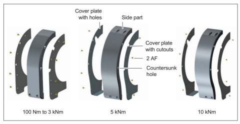
Fig. 8.7 Fitting the cover plates
