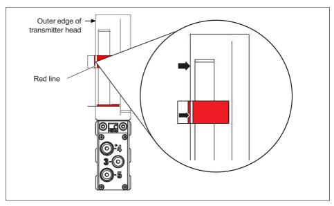
Fig. 8.17 Axial position of the spacers
