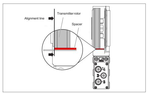
Fig. 8.18 Axial alignment to the rotor
