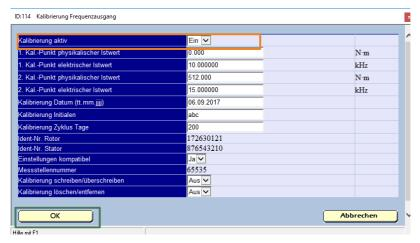
Fig. 14.3 Calibration information for TEDS, frequency output
