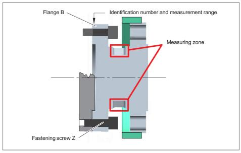
Fig. 8.2 Screw connections, flange B
