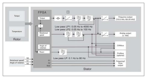
Fig. 6.1 Signal flow diagram
