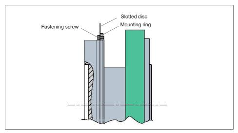
Fig. 8.1 Installing the slotted disc
