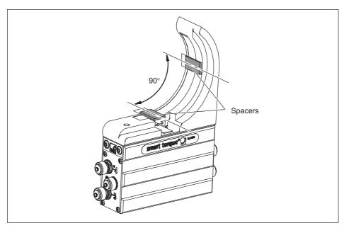
Fig. 8.16 Radial position of the spacers
