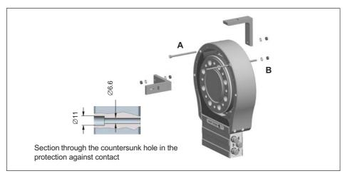
Fig. 8.14 Supporting the stator with protection against contact
