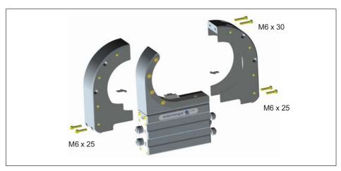
Fig. 8.10 Fitting the two halves of the protection against contact
