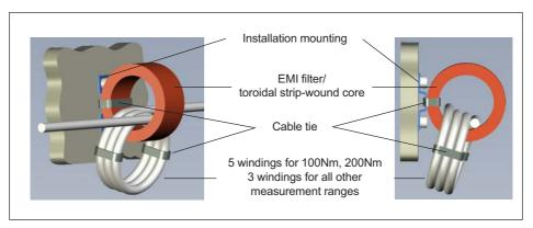
Fig. 10.1 EMI filter/toroidal strip-wound core installation example
