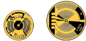
Diaphragm rosette strain gauges
