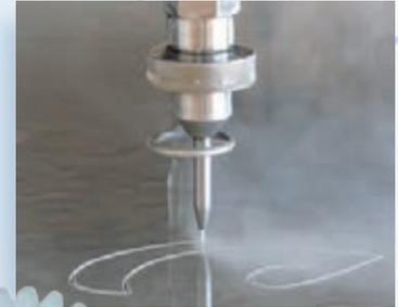
Photo: Water-jet cutting at Döfler
