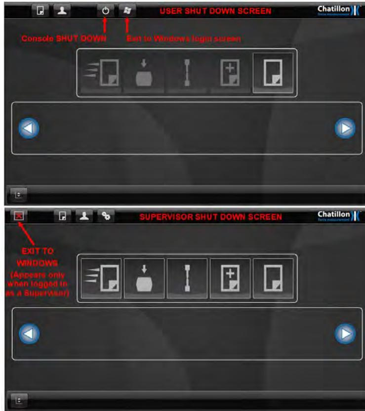
The CS2 tablet should always be shut down FIRST before turning OFF the main power switch. Then the power switch in the rear of the tester may be turned OFF.
