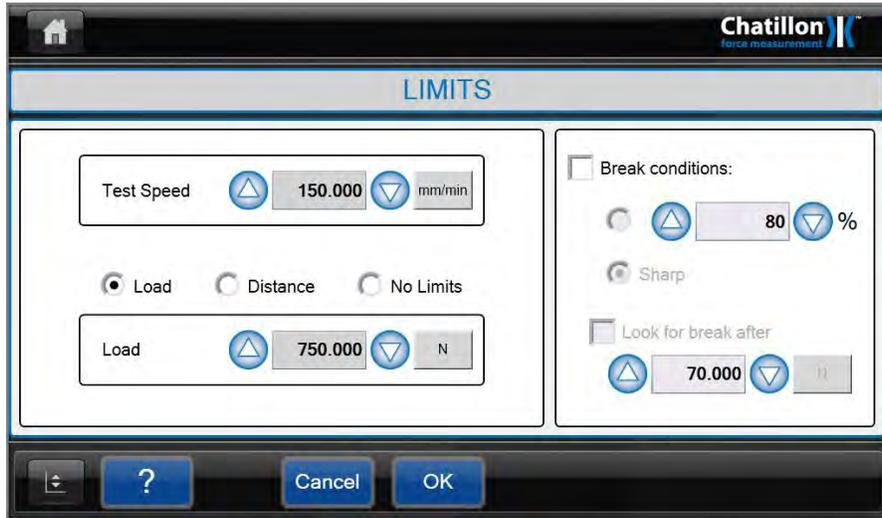
11 Set the Test Speed to the required value (150mm/min in the example screen above), then select the Load option and set the Load to the value required for L2.
