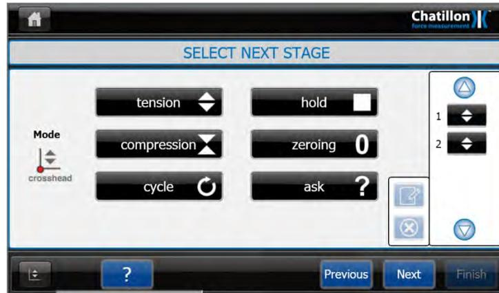
This test action will perform 1 cycle, e.g. move up by 10 inches then move back to the start of test position. Also note that the "CYCLE" button is now enabled.
