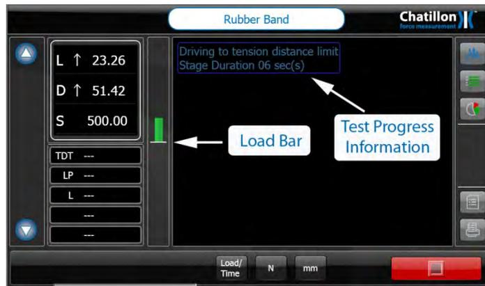
The vertical "Load Bar" indicates the actual load on the Loadcell and will be displayed as a small horizontal line when there is no eye end or grip fitted to the Loadcell.
