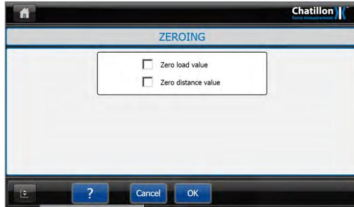
Select "ZERO LOAD VALUE" and / or "ZERO DISTANCE VALUE" as required. Note that the crosshead will stop briefly to allow the system to zero.
