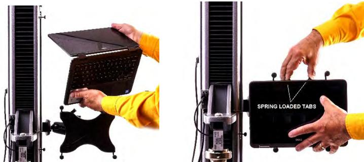
Once fitted, position the Laptop console where it can be easily viewed and operated by the user. Once you have positioned the Laptop console, tighten the hand screw so that the Laptop console is secured in the intended position. Ensure that the control console does not move when pressing on the touch screen.
