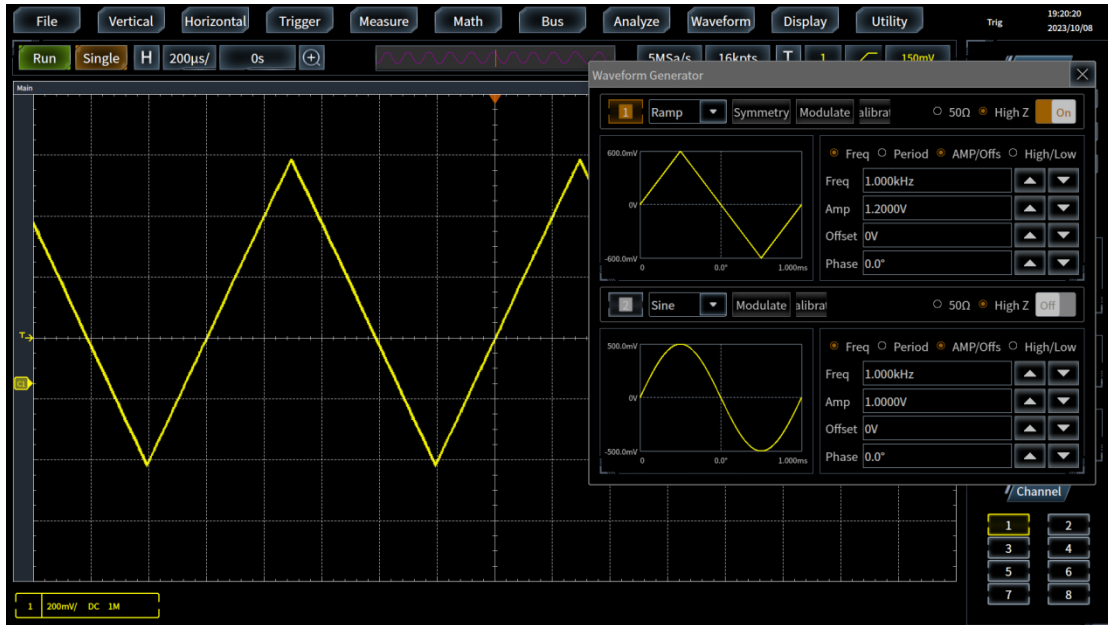
Standard waveform output: sine wave, square wave, ramp, pulse, DC, noise, and arbitrary waves
