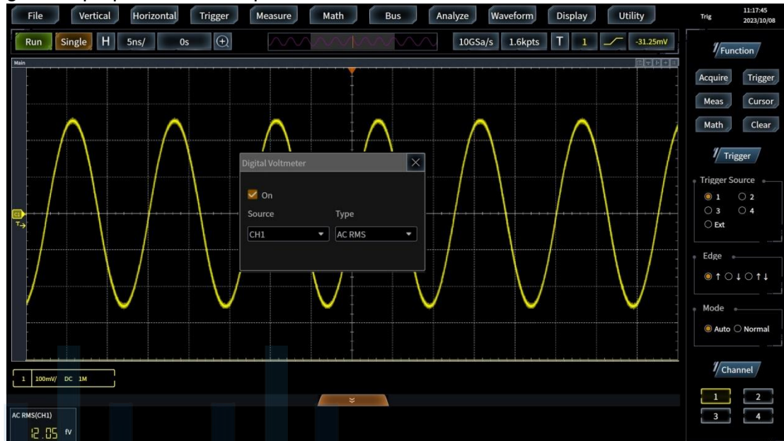
4-bit voltage measurement, 8-bit frequency measurement
