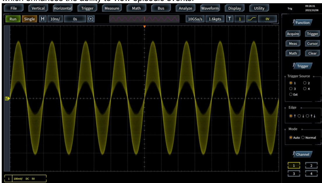
Normal: the default channel color and gray level are used to indicate the probability of an event
