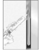
Gun, trowel, or pump approved sealant to minimum 1/4" depth on both sides of wall or top side of floor over the backer rod.
