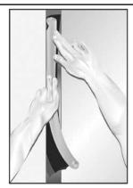
1. Clean all surfaces in joint area to remove loose debris, dirt, oil, wax, grease, old caulking, etc. 2. For floor applications, install a separate base section of backer rod recessed approximately 2" down from the top of floor. Bend and friction fit BIOSTOP® Joint Strip longitudinally into joint using the backer rod as the transport mechanism. Push into joint far enough to accommodate the required depth of caulk.
