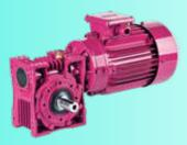
The worm gearboxes of the E series feature input and output shafts that are perpendicular to each other. Their worms are made of steel and gears are made of bronze. They can be mounted to the driven machine by the foot,flange or torque arm on the gearbox.
