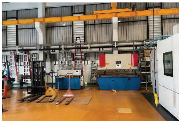
Cutting machine and facility support crane 5 tons
