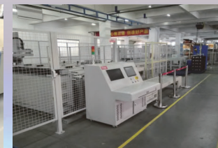
Online lithium cell multi-grade sorting test system
