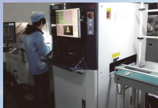
Online 3D SPI solder paste detection system
