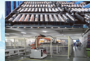
Robot optical positioning laser welding battery core&BMS system
