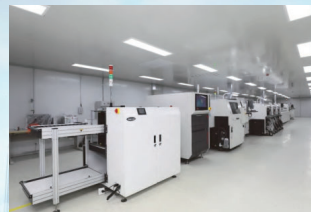
Rotary multi-head high-speed high-precision full automatic SMT machine
