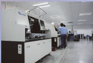
Full-automatic solder paste printing machine
