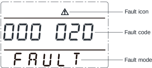
Tower UPS LCD display in fault mode
