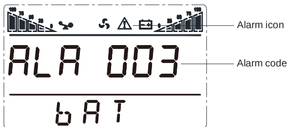
Tower UPS LCD display in alarm mode
