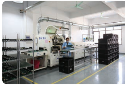
Figure1 Fully automatic coating machine Figure 2 Coated circuit board
