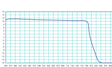
Gain (x: frequency MHz, y: ISO dBi gain) and Pattern (@790MHz)
