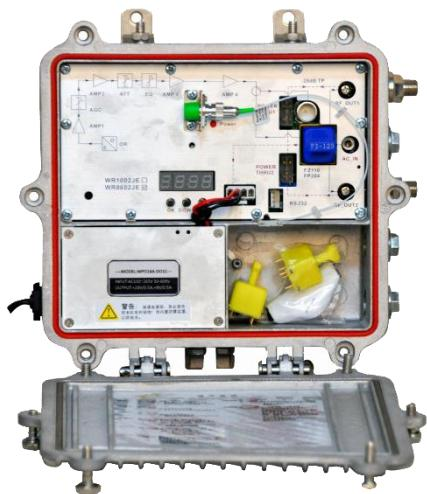
The **ACE WR8602JL** is our new high-class 2-way output CATV optical receiver.
