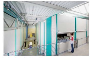
Depending on the height of the Hänel Lean-Lifts®, access points can be installed on different floors. Several people can use the Hänel Lean-Lift® simultaneously at different nositions and levels
