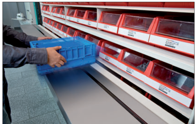
Work counter of high-grade V2A stainless steel
