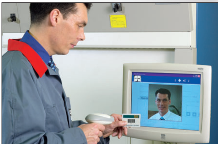
User authentication via ID card, PIN code or RFID transponder
