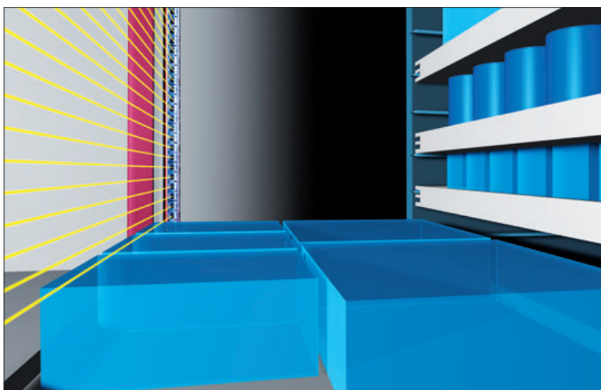
The storage items are measured in the access point by the height sensors
