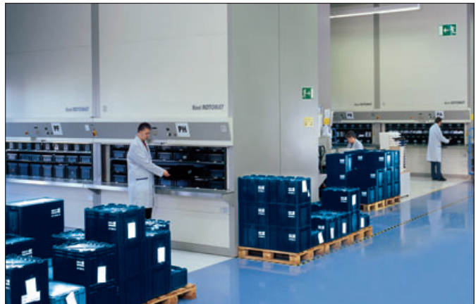
Antistatic storage in the Hänel Rotomat® industrial carousel right at the production line
