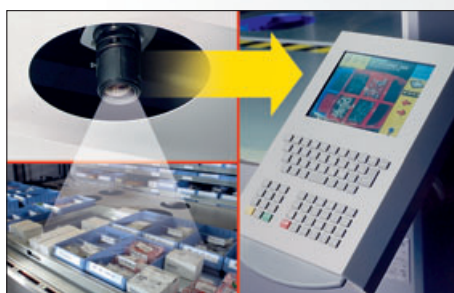
The items are photographed and the picture displayed directly on the control unit
