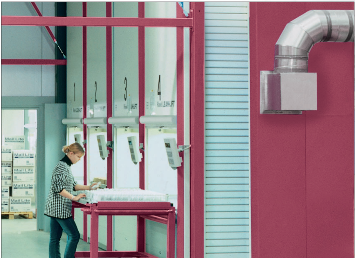
Storage of highly sensitive pacemakers at constant humidity with the Hänel Lean-Lift ® DryStore
