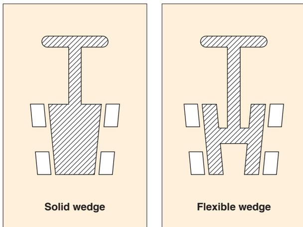
Solidly designed KITZ wedge gates are forged or cast solid, single piece of steel without any welding work. Specially heat-treated wedges are firmly coupled with integral T-head of the valve stems, which are also ruggedly designed and specially heat-treated for the highest possible durability of stem to wedge connection. API 600 Paragraph 5.8.8 particularly emphasizes the importance of the mechanical strength of this connection.
