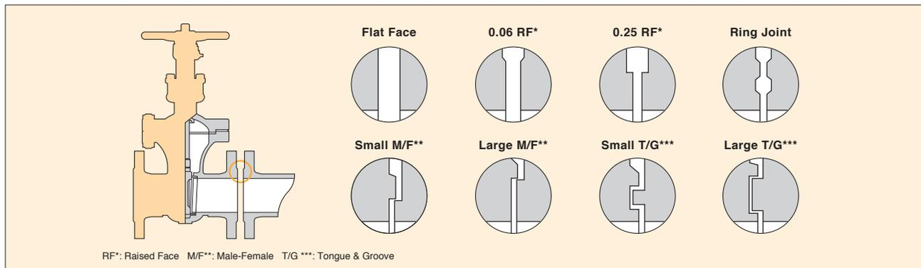
Gasket contact surface finish of end flanges as well as body-bonnet flanges depends on the materials selected for flange gaskets.
