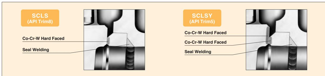
For KITZ cast steel valves made of ASTM A216 WCB, the standard shell material, disc seats and body seat rings are provided as follows. (Refer to Page 02 for Product Coding)
