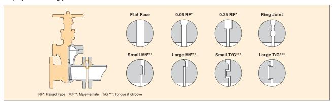
Gasket contact surface finish of end flanges as well as body-bonnet flanges depends on the materials selected for flange gaskets.
