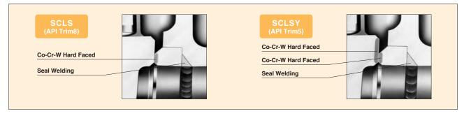
For KITZ cast steel valves made of ASTM A216 WCB, the standard shell material, disc seats and body seat rings are provided as follows. (Refer to Page 02 for Product Coding)
