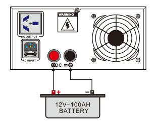
1. 350W/500W/700W/1000W/1200W series wiring diagram
