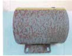
Old : under coat by dipping
