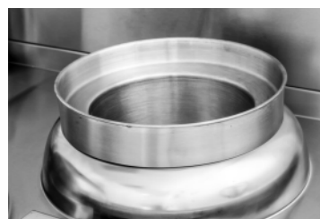
B. Rear Pot for preparing hot water and storage
