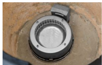
1. Innovation pre-mix burner to reduce combustion noise and enhance efficiency
