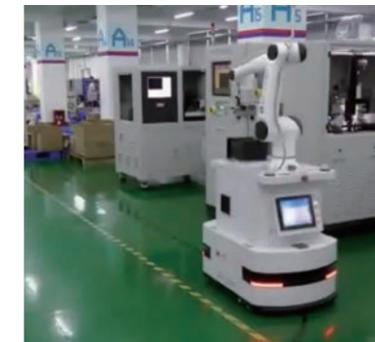
Automatic loading and unloading on the dicing and splitting machine
