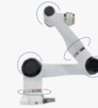
Each joint with a motion range of  $\pm 360^\circ$
