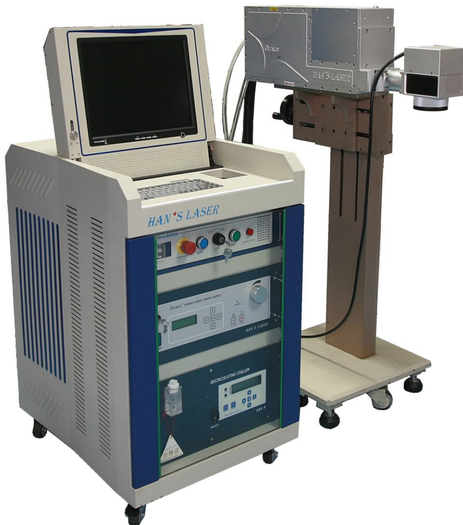
Standardly-configured HLT-EP30 Laser Marker
