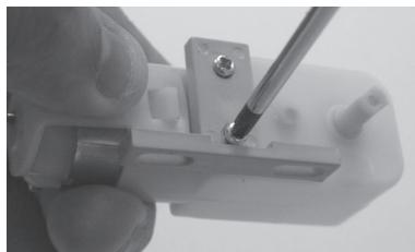
Take off the both screw of motor gear and then mount the motor lock.
