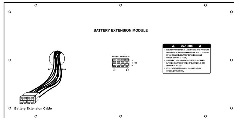
Battery Extension Module, Rack Mount Type
