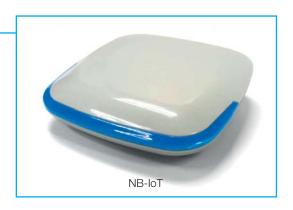
Leonics NB IOT is Low Power Wide Area (LPWA) technologies developed for IOT application with low bandwidth cellular communications. All devices such as UPS, battery monitoring or solar power power system can connect with NB IOT to transmit data to cloud server by using TCP protocal with low power consumption.
