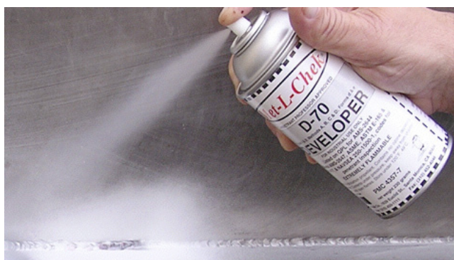
Typical aerosol application of D-70 during a weld inspection.
