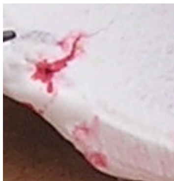
Visible penetrant crack indication on D-70
