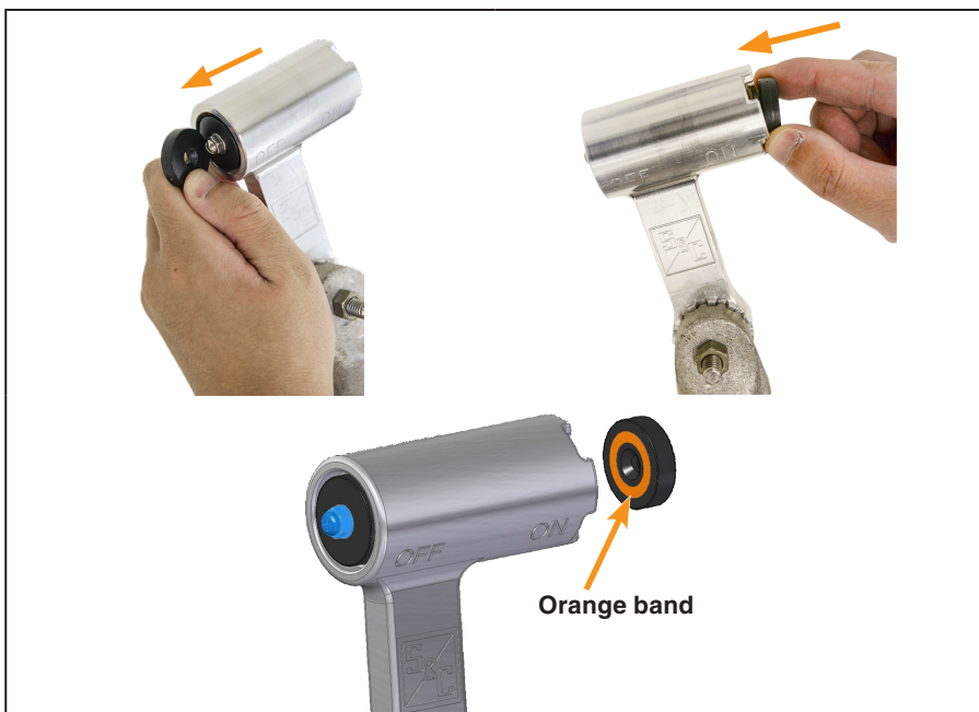
Figure 2. Moving the magnet to the “ON” side of the tool.
