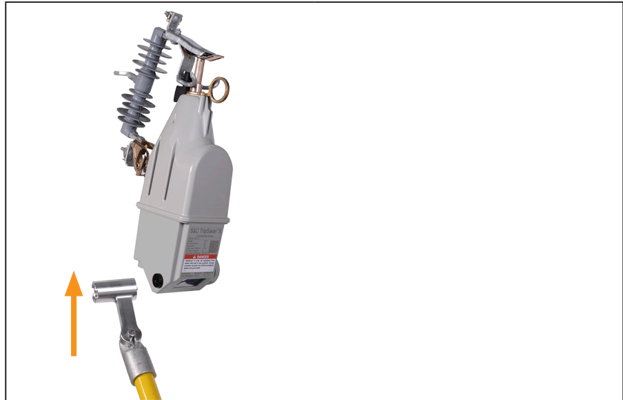
Figure 6. Flipping the magnet tool and raising it up.
