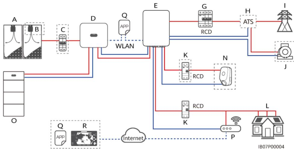
**Figure 2-5** Networking with some of loads connected to the SmartGuard (dashed boxes indicate optional components)
