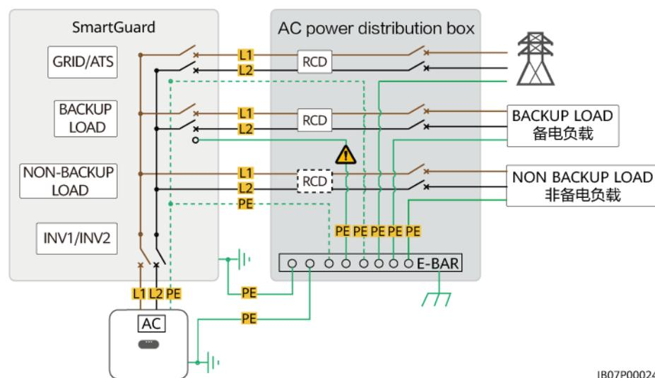
**Figure 2-3** SmartGuard-63A-AUS0 residential wiring diagram (dashed lines indicate optional cable connections)
