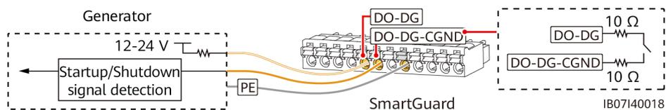
**Figure E-2** Generator alarm signal
