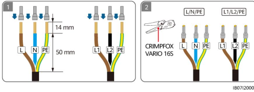
**Figure 5-18** Crimping SmartGuard-63A-AUS0 AC cord end terminals
