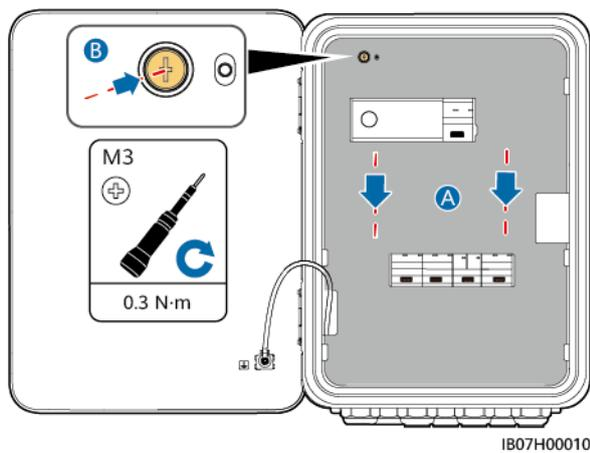
**Step 2** Before closing the maintenance compartment door, turn on the three switches shown in the following figure (using the connection to the LC0 inverter as an example). During deployment and normal operation, do not operate the bypass switch shown in the figure.
