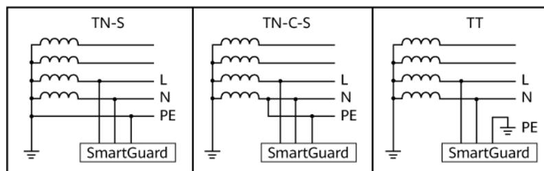
**Figure 2-8** Earthing system (L1/L2 dual-live-wire connection)
