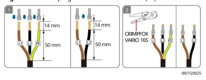
**Step 2** Connect the non-backup load output power cable.
