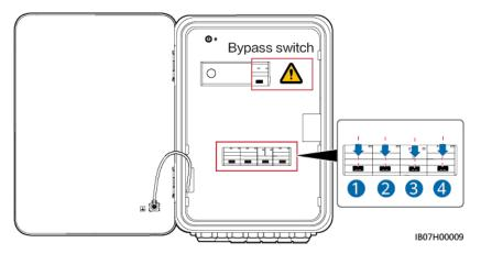
**Step 3** Remove the screw from the maintenance compartment cover, and open the cover.
