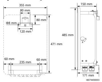
Figure 4-1 Mounting bracket dimensions
