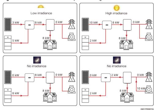
Figure 2-6 Illustration of maximum power in off-grid mode
