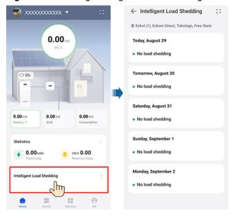
Figure F-3 Viewing intelligent load shedding
