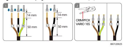
**Step 2** Connect the inverter AC input power cable. Currently, only one inverter can be connected to the SmartGuard. Select a port based on the inverter model.
