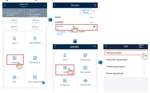
Figure 6-7 Setting the output mode
