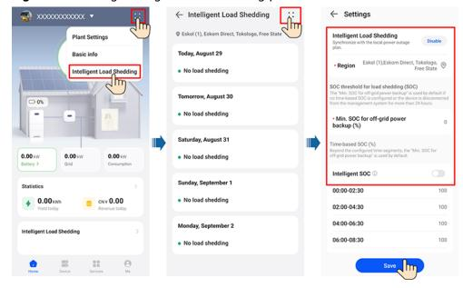
Figure F-1 Setting intelligent load shedding parameters
