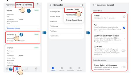
Figure F-4 Generator control settings
