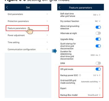
Figure 6-6 Setting off-grid mode
