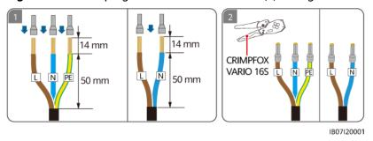
Figure 5-14 Crimping AC cord end terminals (L1/L2 dual-live-wire connection)
