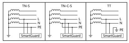
Figure 2-8 Earthing system (L1/L2 dual-live-wire connection)
