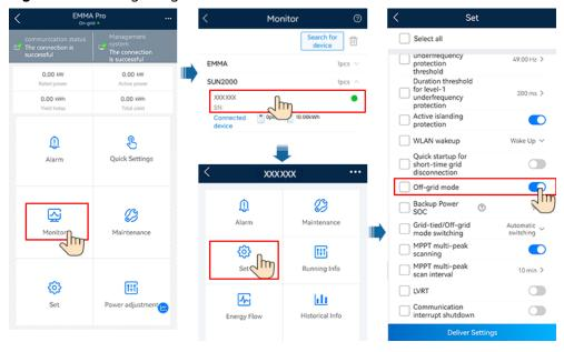
Figure 6-5 Setting off-grid mode
