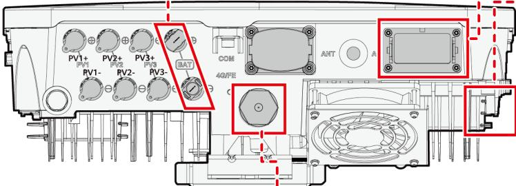
**EN-GB** Installing the Smart Dongle
