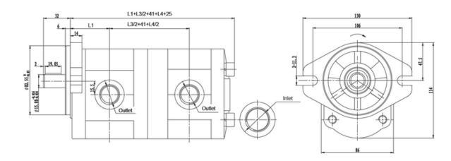
A double aluminum gear pump consists of two gear pump sections combined into a single housing, usually made from lightweight aluminum alloy. It is used to generate hydraulic pressure and flow in systems requiring multiple outputs or circuits, such as in construction machinery, agricultural equipment, and industrial hydraulics.
