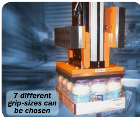
UniGripper WingGripper for picking of single SKU's into mixed pallets.
