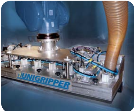
UniGripper with 8 controllable zones for effective palletising and pattern build.
