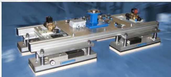
Special-tool with 4 SMS-grippers for bread-handling
