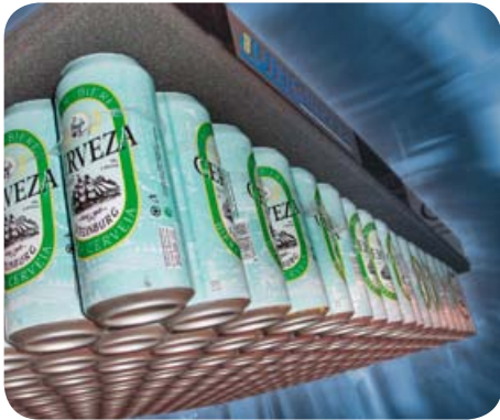
UniGripper for handling of cans, filled or empty, single or shrink wrapped.
