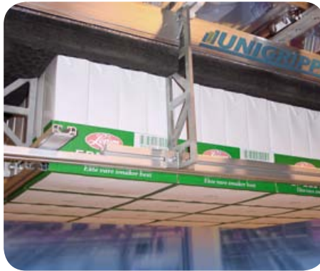
UniGripper for handling of packages with loose trays or shrink wrapped.
