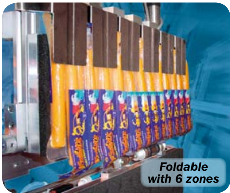
UniGripper custom built for handling of cheese-strings packages.
