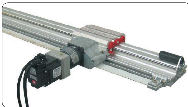
Motore Mitsubishi Mitsubishi motor HF-KE23BW1-S100 (200W) (non fornito) / (not supplied)
