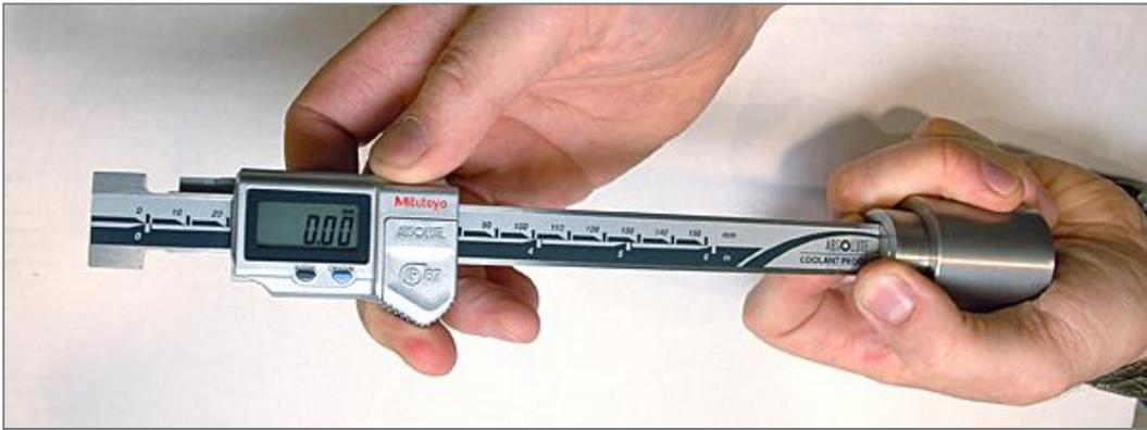
Hold the gauge boss tight into the reference block and move the digital display towards the reference block until the contact rests on the datum point.
